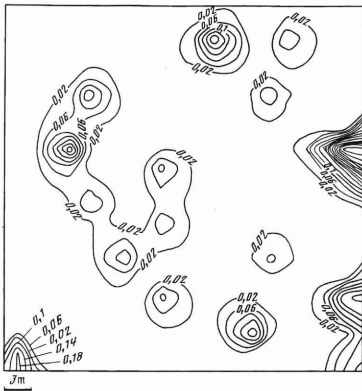
Fig. 49. Spatial distribution of ^{144}\text{Ce} in the upper 10 cm mineral soil layer ( \text{Ci}/\text{km}^2 , 5 km from ChNPP)
